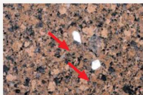
Contamination caused by iron.
