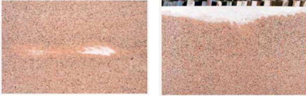
Non-conforming Polished surface with paper Fissure in the polished slab.
